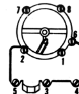
AIR HORN TIGHTENING SEQUENCE
